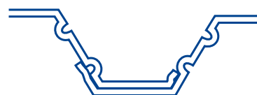
Detalle de solape / Overlap detail Medidas en mm. / Measurements in mm.
